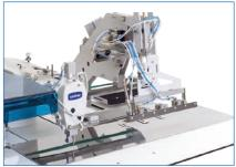
The OZ 5400-IX is a sewing machine with which all straight facing can be stitched efficiently and with good stitching quality on pocket pouches. Different top stitch width can be adjusted by an efficient folding device. The program enables sewing over the entire length of the pocket pouch as well as sewing only over the length of the facings.
