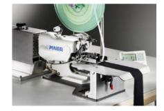
High-performance blind stitch sewing machine MG 2000 for the fabrication of double-folded belt loops with inserted tape and loops for neckties. The sewing machine is equipped with a front cutter which cuts any material remnants to the needed width for the folder integrated in the machine. Two upper feed dogs, one in front and one behind the needle, take care for a perfect feeding process.
