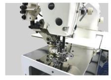
The WX 3100 with integrated direct drive offers a first-class solution for stitching waistbands of skirts and trousers in seam shadow. The combination of bottom, top puller feed and sewing equipment, specially developed for this work sequence, makes it possible to process waistbands accurately and true to shape.
