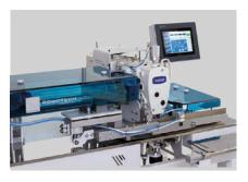
Automatic short seamer QX 9400-IX is for darts and waistband pleats. Darts and pleats play an important role for the fit and for the overall visual appearance of trousers. Consistent quality and economic processing on a machine that is easy to operate. The QX 9400-IX short seam automatic sewing machine meets this requirement.
