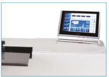
The ID 4400 INDEXER produces a buttonhole which has a similar appearance to a normal buttonhole but is purely decorative and non-functional. This type of buttonhole is not cut and is used on the sleeves of men's and ladies' jackets, suits and sports coats. Since this buttonhole is not cut, and is done on a fast chain stitch machine, sewing at speeds up to 3,800 spm, the operator is able to sew 2-3 times more jacket/coat sleeves, than with a conventional buttonhole machine.
