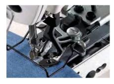
Oil-free, clean and durable machine thanks to the black diamond bar thread pick-up lever and the micro-oil lubrication system direct to the rotary hook. Fabrics are prevented from oil stains.
