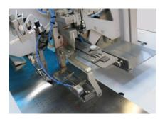
FF 6200-PTO is a dedicated sewing unit for slanted Breast Pockets on Men's Jackets ONLY! The PTO version is equipped with matching device for chequered or striped fabrics; with automatic adjustment of the corner knives as to the breast welt angles. The unit provides maximum speed and quality compared to manual sticking of the breast pockets.
