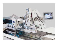
The sewing system OZ 7300-IX is designed for small to medium size trouser production facilities. Besides felling pocket facings on pocket pouches, the left fly piece can be felled and the right fly piece can be felled on and even the right and left pocket facings can be felled at the opening. Wing pocket top stitching is another operation area possible whit this unit.
