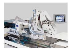
Sewing system OZ 6300-IX for felling and sewing the fly pieces. The sewing unit offers an excellent solution for this production. With the OZ 6300 - IX you can sew:  $\cdot$  the left fly  $\cdot$  the right fly
