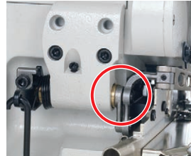
<Presser arm shaft at its upper position>
