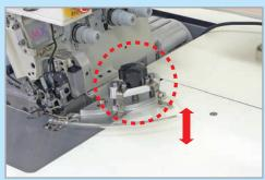
The guide height can be adjusted effortlessly according to the fabric thickness.
