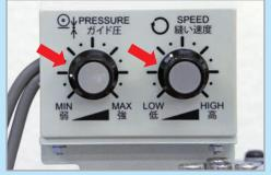
The machine speed and the edge controller pressure can be readily adjusted with the knobs placed at the front of the machine.
