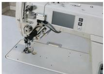
GM 5100 Single thread blind stitch sewing unit for fusible coated tape. Fusible tapes coated on one side can be attached to jacket fronts or facings to be fused to the jacket. In spite of a low work input this semi-automatic unit guarantees high quality combined with high efficiency. The machine is equipped with a tape feeding device, tape cutter, thread trimmer and the option to predetermine the seam length. The tape feeding device guarantees reliable tape feeding.
