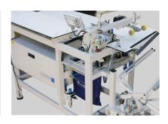
Automatic serging of denim trousers. The sewing unit D-SS 430-G1 with Pegasus EXT 5214 offers excellent solutions for the rational serging of front and hind denim trousers parts. This automat has especially strenghthened feeding and puller mechanisms as well as heavy duty stacker for denim fabric weight.
