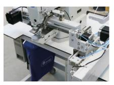
Satin and nylon hanger loop attaching automat with auto cutter and adjustable loop length system.
