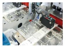
The machine is used for automatic joining of up to 8 care labes from label rolls.
