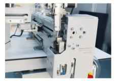
Satin and nylon hanger loop attaching automat with auto cutter and adjustable loop length system.
