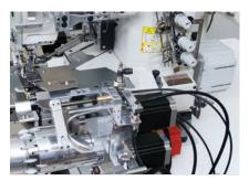
PE 6000 is an automation for folding and hemming on skirts of T- shirts, underwear and similar garments. This automat improves speed, stich quality and consistencey. It saves time and labor since operator can use two machines simultaneously. Sewn garments are automatically stacked after the sewing cycle
