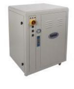
**TYPE** HSL-MK-20 400 V ~3 Voltage NPE Frequency 50 Hz **Total Power** 20,55 kW Power Of Pump 0,55 kW Power of 2\*10 kW Resistance **Working Pressure** 4 bar Water Tank 50 lt 67\*57\*100 Dimensions cm
